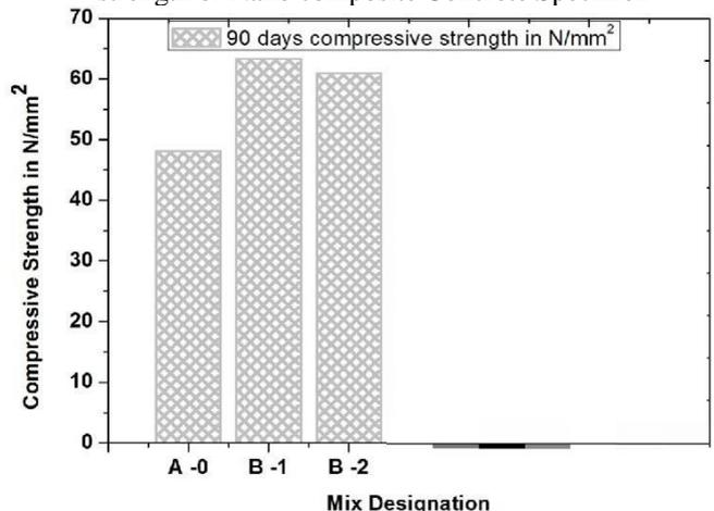
Figure 4.14 90 Days compressive strength of nano composite concrete specimen.
