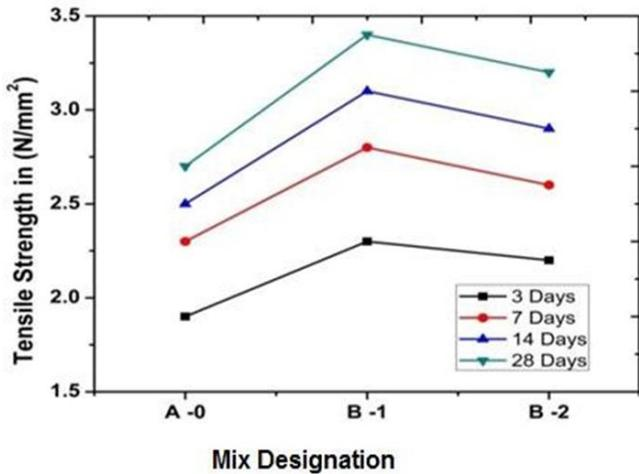
Figure 4.15 Variation of binary combination of tensile strength of control and Nano Composite Concrete Specimen B-1 and B-2 mix.
