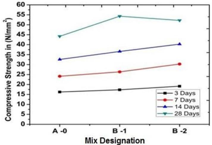
Figure 4.12 Variation of binary combination of compressive strength of control and Nano Composite Concrete Specimen B-1 and B-2 mix.
